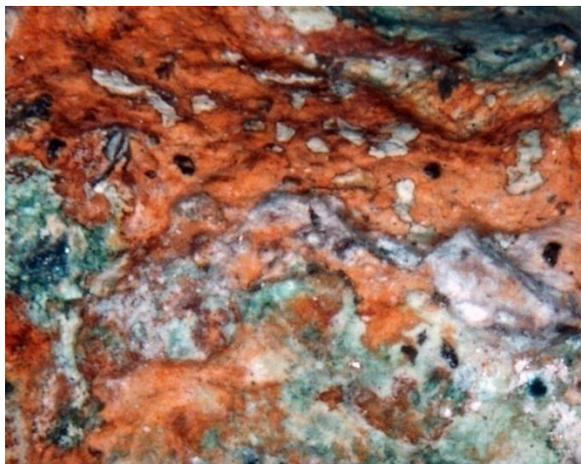
*Fig.1b: The 3D video microscopic image of the concretion and corrosion on the surface of the copper coin.: (X. Tian).*
