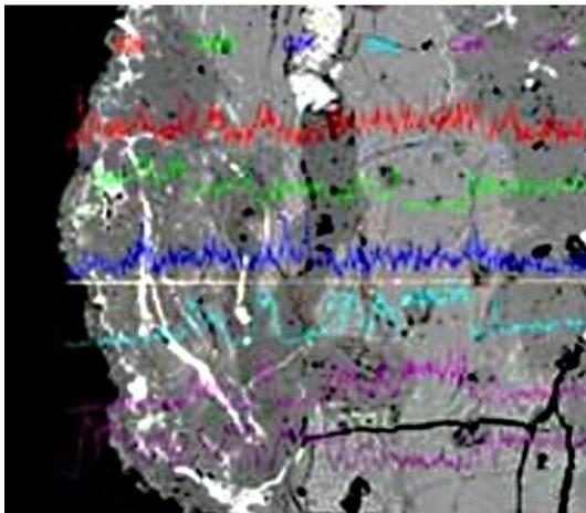
Fig.4: The content line of different elements in the cross section of the copper coin.: (X. Tian).
