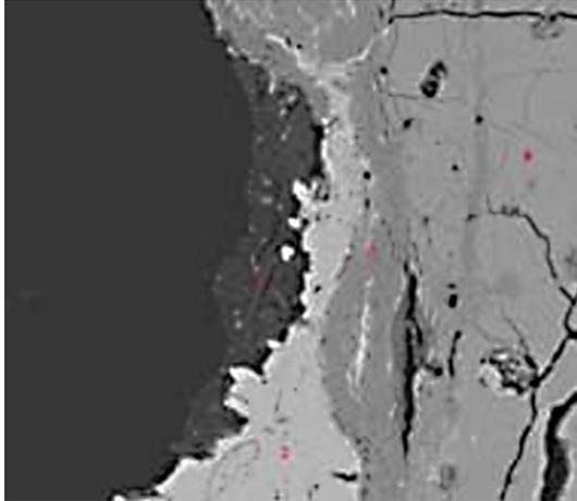
Fig.3: SEM image of the cross section of the outer layers of the copper coin.: (X. Tian).
