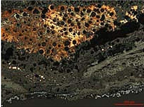
Fig.1c: The metallographic dark field image of the cross section of the copper coin.: (X. Tian).
