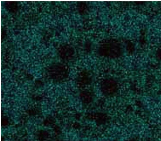
Fig.2d: distribution image of Sn.: (X. Tian).
