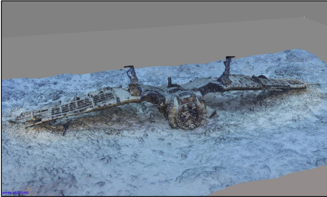
Fig. 3: Photogrammetric model of the Vought F4U Corsair at Midway Atoll (Image courtesy of Bert Ho, Exploring the Sunken Heritage of Midway Atoll expedition 2017).
