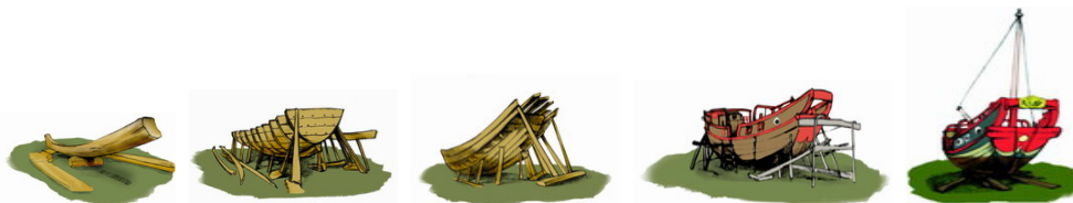
Figure 2. The sequence of construction.
