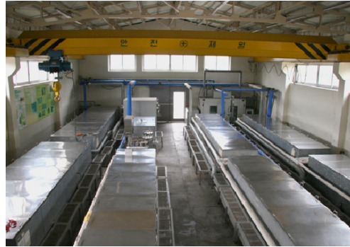
Figure 2. PEG treatment tanks for salvaged ship (NRIMCH)
