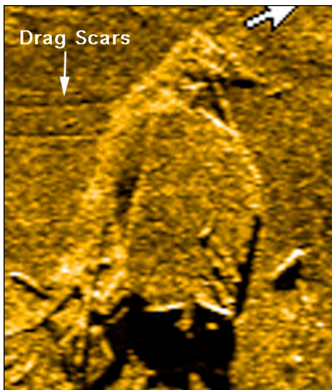
Figure 100. 2003 acoustic image of the East Casemate section. When compared to Figure 99 above, the damaged areas as well as the linear drag scars are clearly evident.
