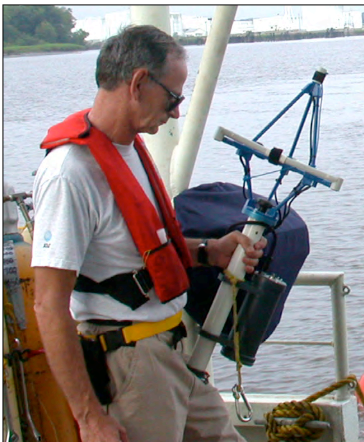
Figure 24. Photograph of the Aqua Metre D100's ultra short baseline transducer array that was positioned at the start of the dive on a selected datum.
