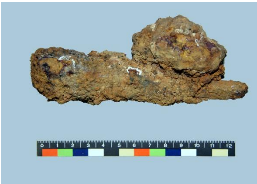
Fig. 5 Iron nail from the South China Sea I shipwreck. (a) Before deconcretion, (b) After concretion removal. (Z. G. Zhang)
