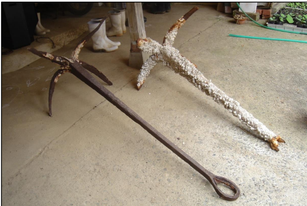
Fig. 4: Iron Grapnel Raised up off Suzu City, Ishikawa Prefecture. Although sometimes it displays slight lamellar traces and forge contact traces due to forge weld, surfaces of Japanese iron grapnel are flat.
