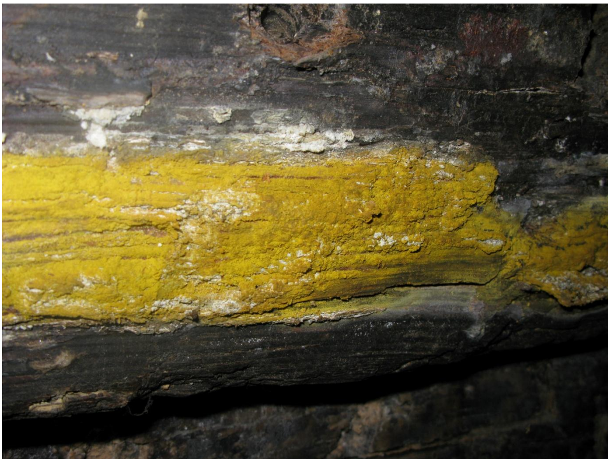
Figure 2. Acid-affected region on a hull timber of the Shinan ship (Copyright: National Research Institute of Maritime Cultural Heritage, Korea).
